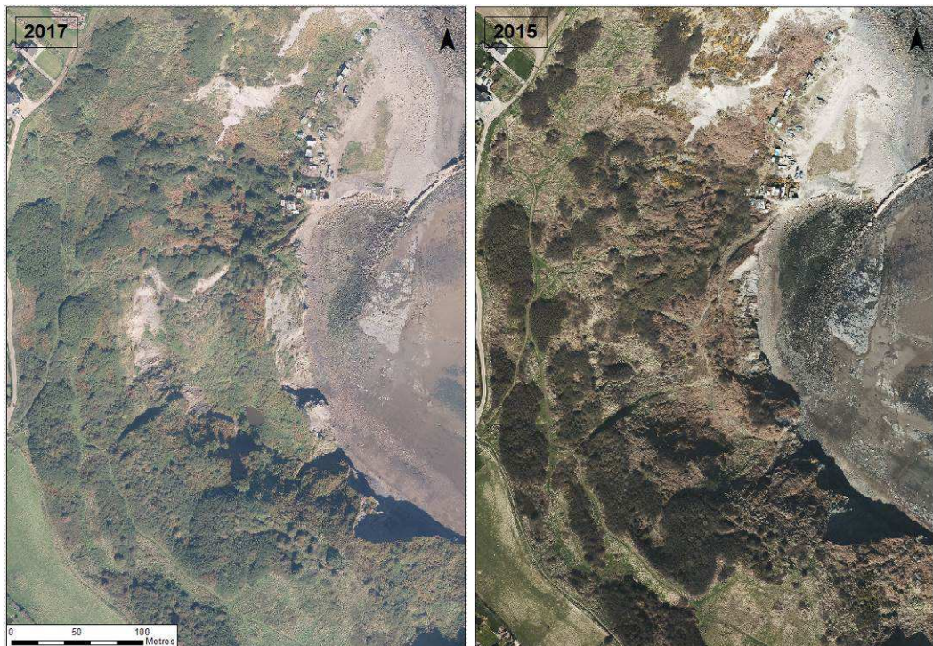
Figure 2-14 – Large landslip within Port Mulgrave
