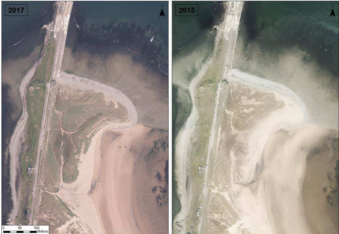
Figure 2-5 – Vegetation growth on dunes in the lee of South Gare Breakwater
