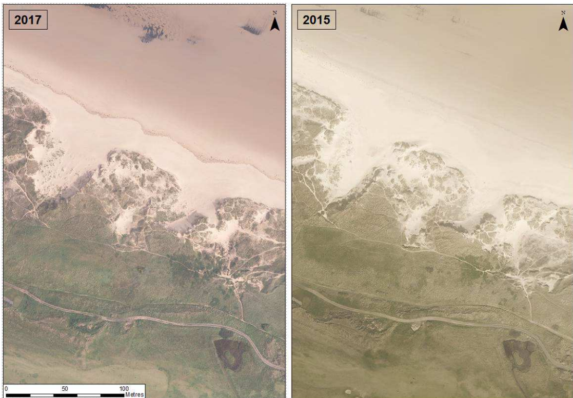
Figure 2-8 – Damage to dunes along Coatham Sands pre-dates January 2017 storms
