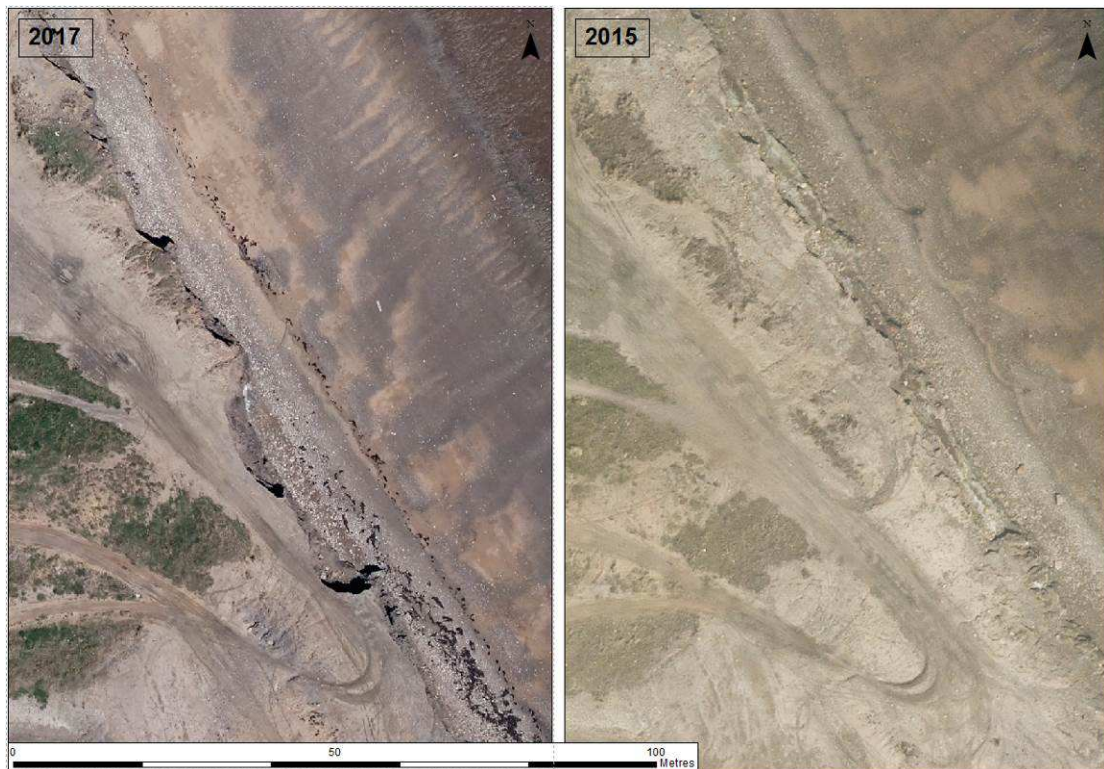
Figure 2-4 – Erosion of colliery spoil south of Lynemouth
